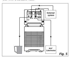
**Note:** When the external system is not necessary, please seal the pump connection **IN** and **OUT** with the existing union nuts and stoppers.
